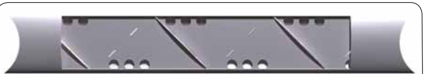
Oval tube detail with cut-away showing the MPADVANTAGE™ HelyX insert, patent pending
